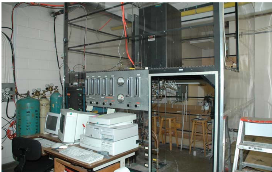
Figure 7. High temperature reactor system for carbon nanotube growth
