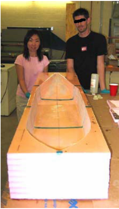
Fig. 7 A CNC-machined foam mold and the thin, light carbon-epoxy fuselage
