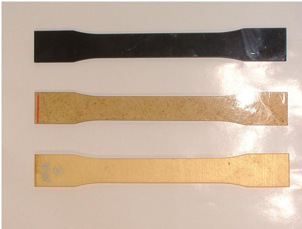
Figure 5. Test specimens with various concentrations of carbon nano tubes.
