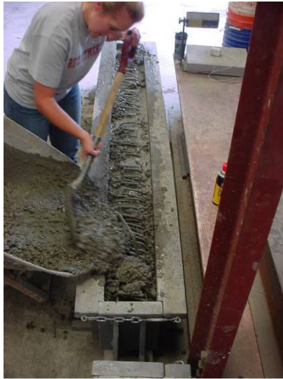
Figure 3. Placing Concrete into Form.
