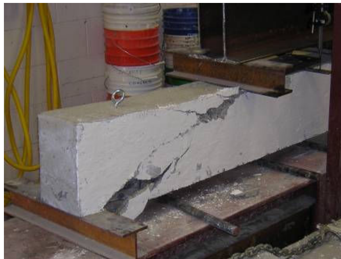
Figure 5. Beam After Testing.
