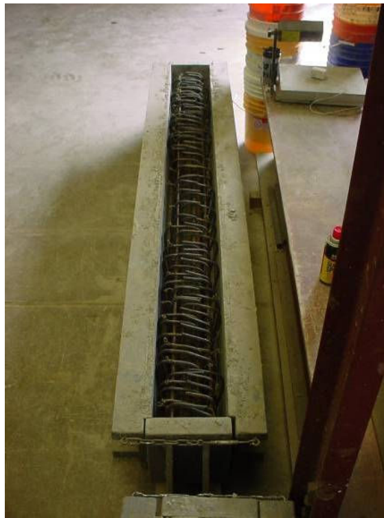
Figure 2. Wood Form Prior to Casting.
