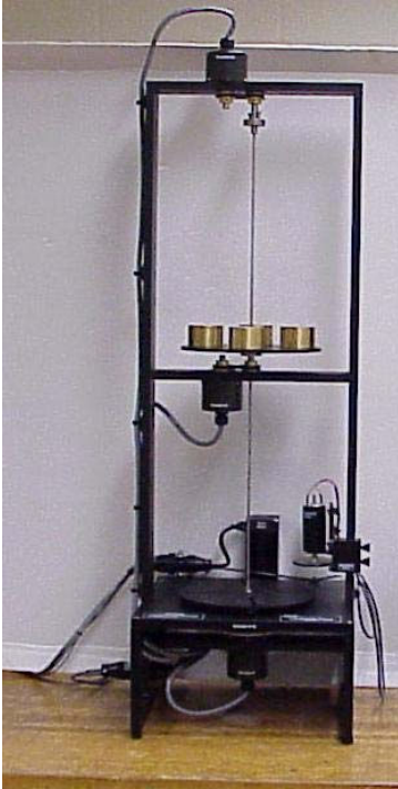
An unrestrained torsional mechanical system
