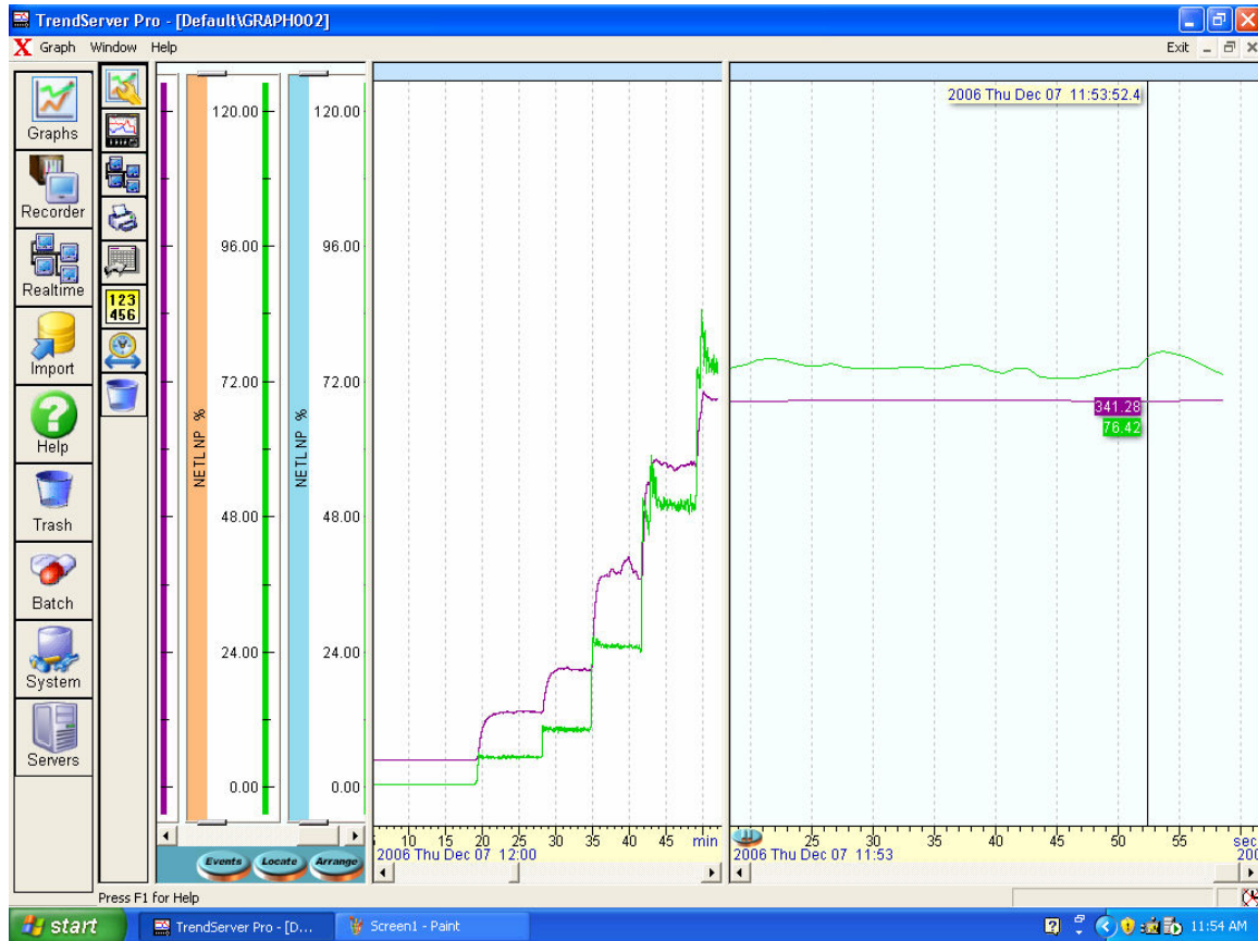
Figure 1. Display shown in classroom. It shows reactor power (% power) and fuel temperature (°C).
