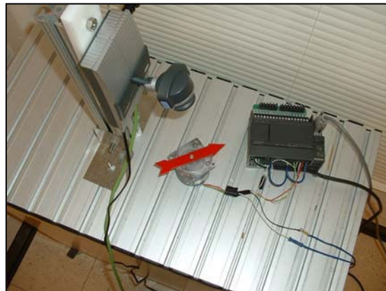
Figure 5: PLC Controlled Stepper Motor Work Station
