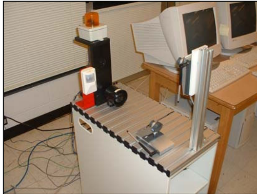
Figure 4: PLC Controlled Alarm Work Station
