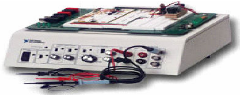
Figure 6: NI -ELVIS and Decade Counter Interface
